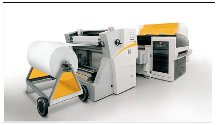
Zimmer offers the complete COLARIStechnology along with the know-how used for operation. Production capacity up to 480 m2/h for the printing width of 180 cm; (per hour 260 linear meters)
