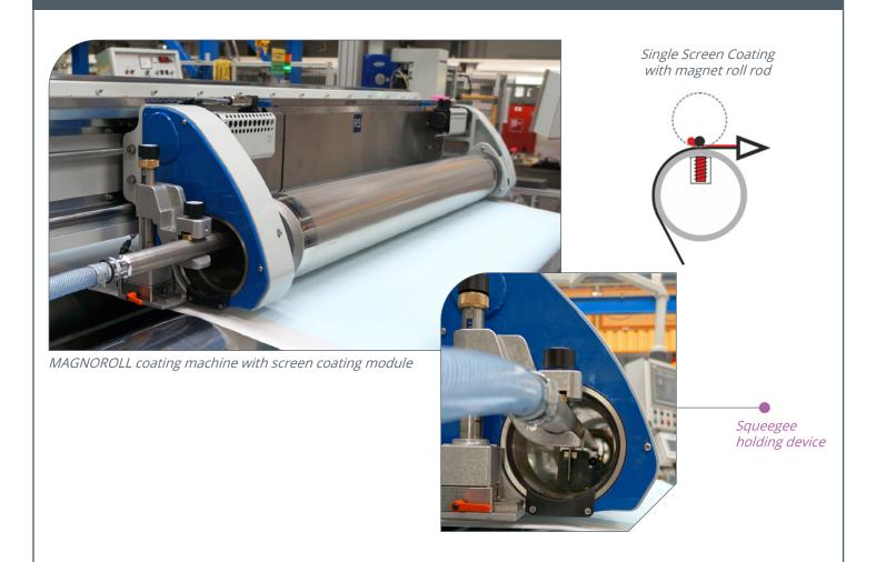
The MAGNOROLL machine can be optionally equipped with two rotary screens for simultaneous application.
