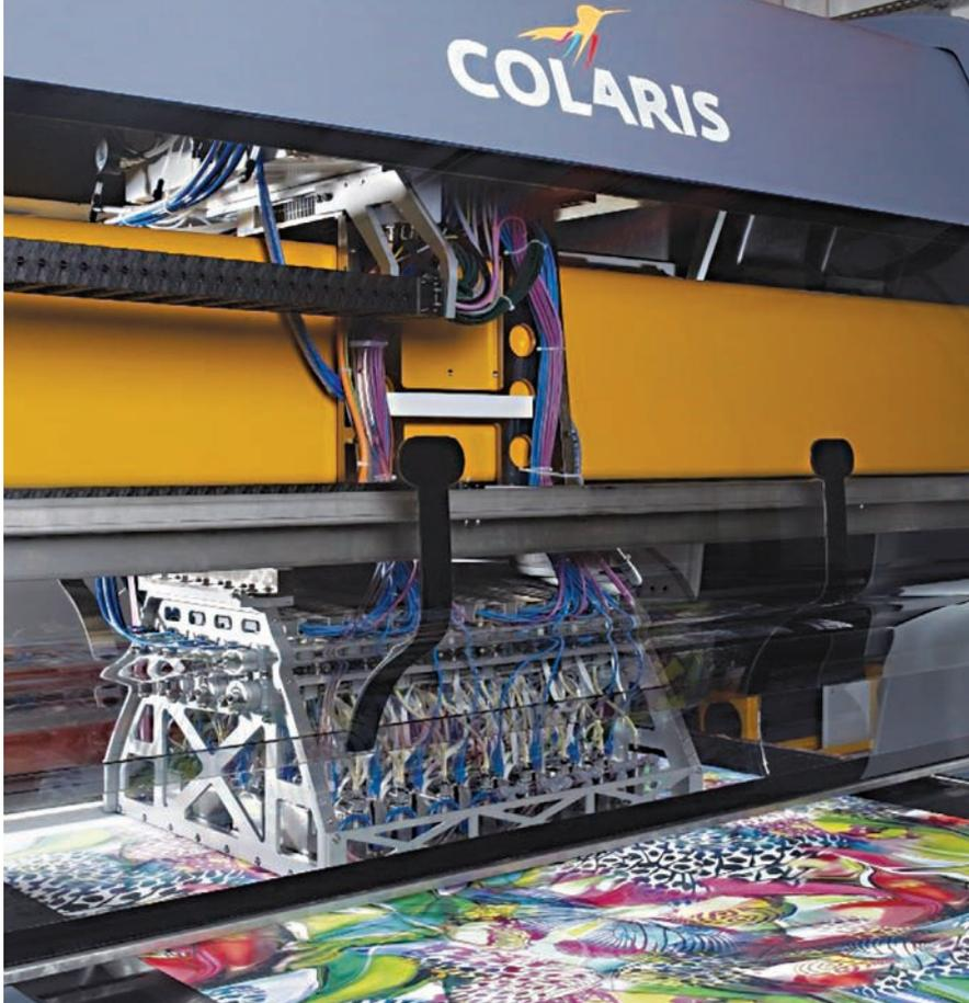
The Colaris series of printers from Zimmer Austria Inc. are compatible with a variety of colorants including reactive, disperse, acid, pigment and vat.
