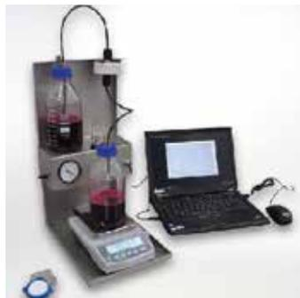
Ink Filtration Tester - to check filterability of ink. The decrease of flow rate is measured over time to see how an ink performs during filtration.
