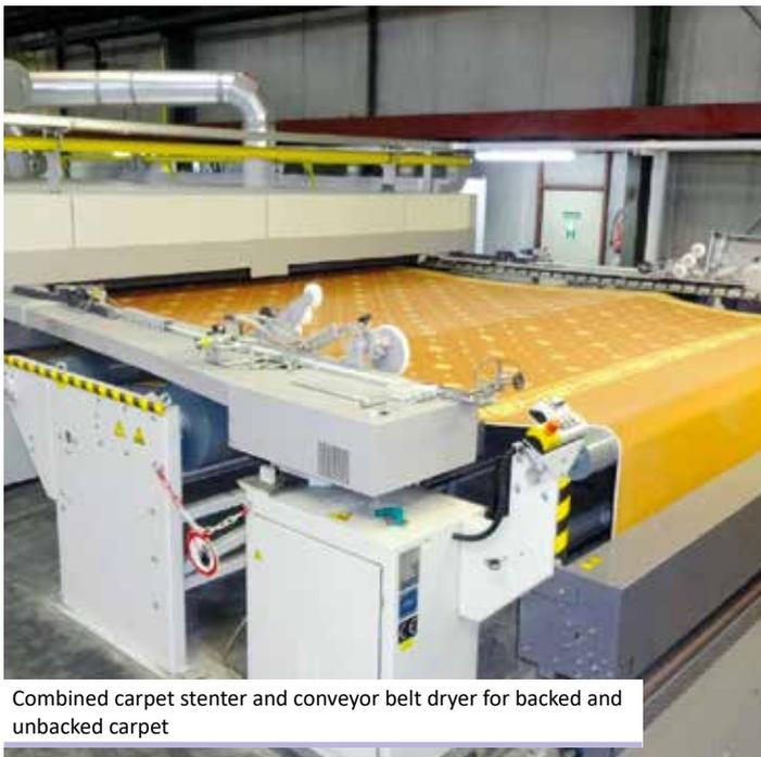
Combined carpet stenter and conveyor belt dryer for backed and unbacked carpet
