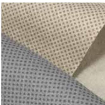
Pigment printing for automotive applications: headliners, insulation layers etc.
