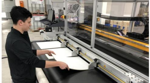
Tile and mat positioning device - which allows to position tiles precisely over the width. The 'fingers' can be adjusted to allow any size of piece good to be printed.
