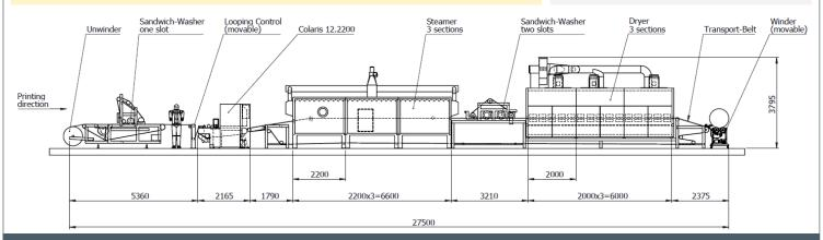
Depending on requirement - **ZIMMER AUSTRIA** builds tailor made print lines based on latest process know-how. *The layout proposal above is only an example how a COLARIS carpet-tile print line could look like.*
