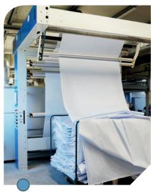
**9** | The COMPACT.HC dryer with an operating temperature of 90°C to 200°C is available on ground floor level or elevated on a substructure. With optimized interior geometry for high energy efficiency and uniform chamber temperature. Self-monitoring and state-of-the-art measuring and regulation techniques. (For more details please see our seperate dryer leaflet)
