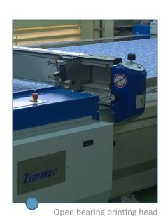
4 | RSDM-V open bearing printing head with colour trough.
