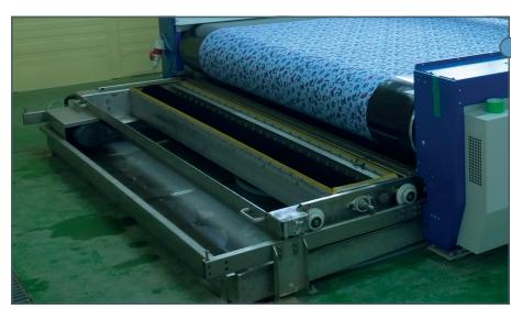
6 | Midi-II washing device with high quality rotating brush, drying squeegee and pneumatic lifting device.
