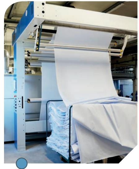
**9 |** The COMPACT.HC dryer with an operating temperature of 90°C to 200°C is available on ground floor level or elevated on a substructure. With optimized interior geometry for high energy efficiency and uniform chamber temperature. Self-monitoring and state-of-the-art measuring and regulation techniques. (For more details please see our separate dryer leaflet)
