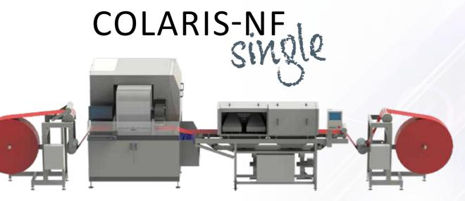
The COLARIS-NF Single is a single-pass digital printer for one-sided printing on narrow fabrics. Onesided printing is typical for individualizing consumables such as face masks or cleaning wipes. It is also used for printing on hook & loop quick-fix-and-release tapes, bandages or decorative tapes.
